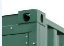
International Standard Twist-lock Corner Fittings
